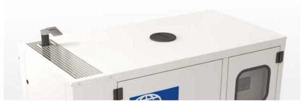
The robust single piece roof incorporates a flush mounted access cap with compression seal, allowing access to the single point lift, whilst providing excellent protection against water ingress. The exhaust silencing system is housed inside the enclosure, delivering market leading noise levels while ensuring operator safety.
