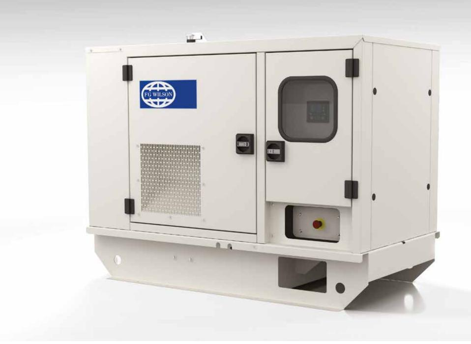
This range of enclosures offer excellent service and maintenance access. The control panel tower mounted on the side of the generator set is accessed via the full height door, allowing access to the control panel including all components and wiring. Side hinged doors open to 180° and can be lifted off when opened at 90°. Combined with removable front and rear access panels, the enclosure provides optimal access for all servicing and maintenance tasks.
